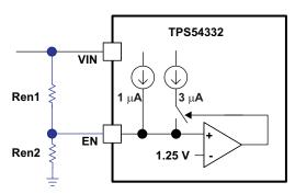
Figure 11. Adjustable Input Undervoltage Lockout
