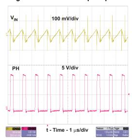
Figure 21. TPS54332 Input Ripple
