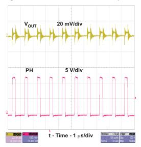
Figure 20. TPS54332 Output Ripple
